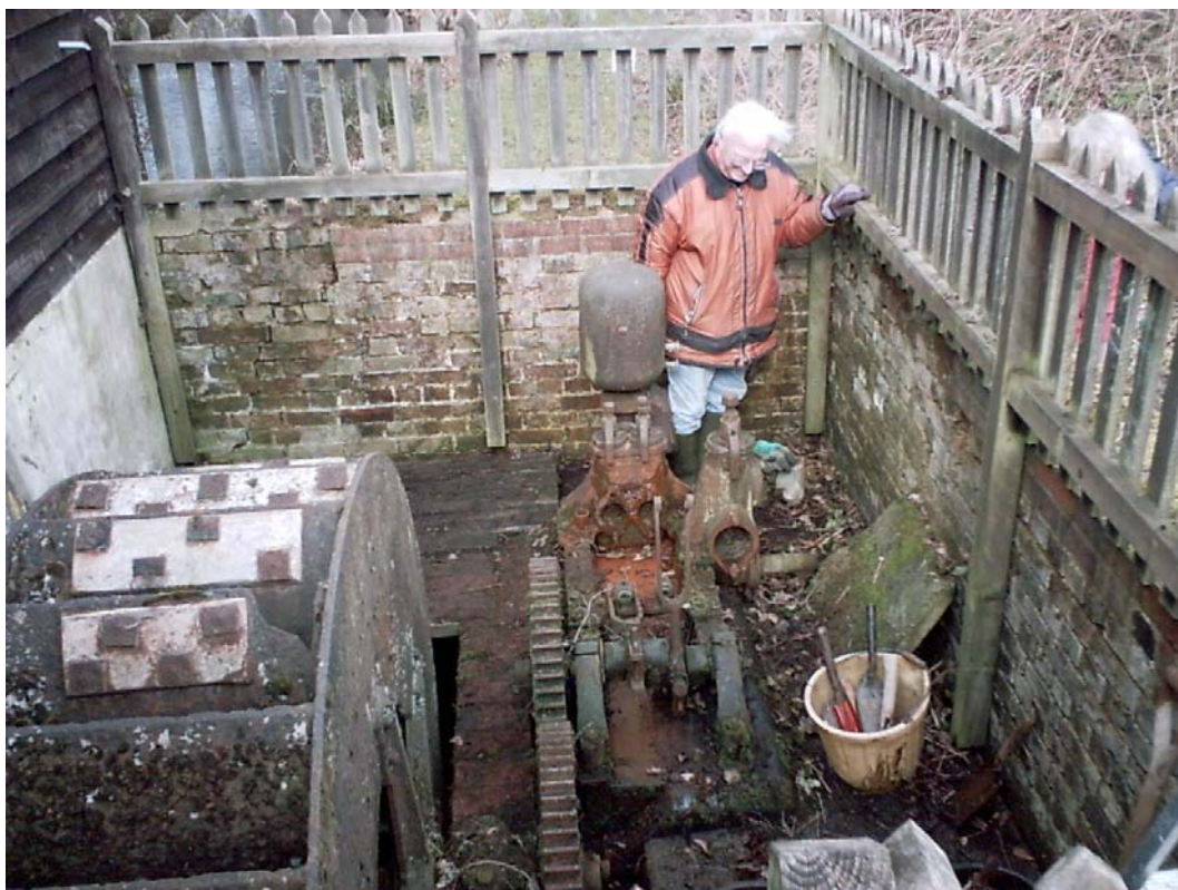
Before and During Clearance of Vegetation (The rivetted-on plates were probably for adjusting the balance)
