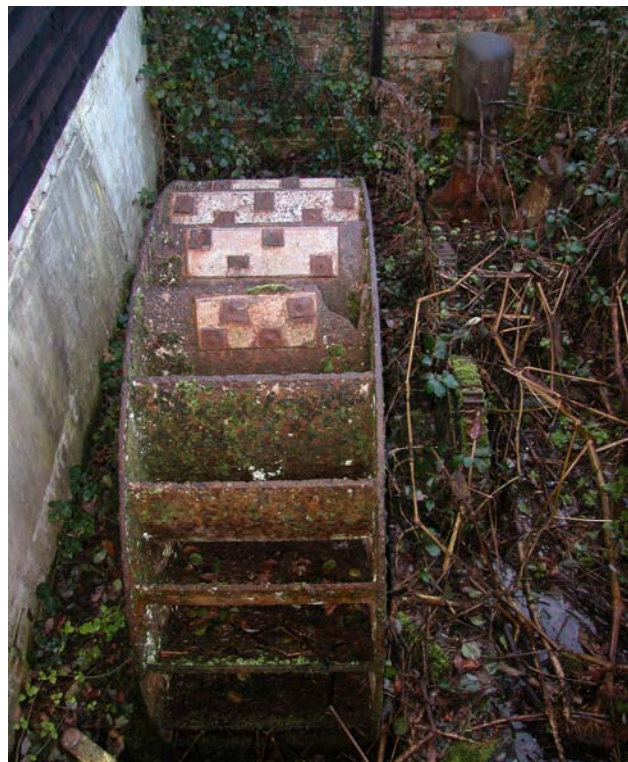
Before and During Clearance of Vegetation (The rivetted-on plates were probably for adjusting the balance)
