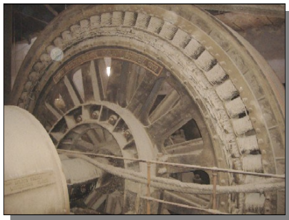
MAN generator coils incorporated in flywheel
